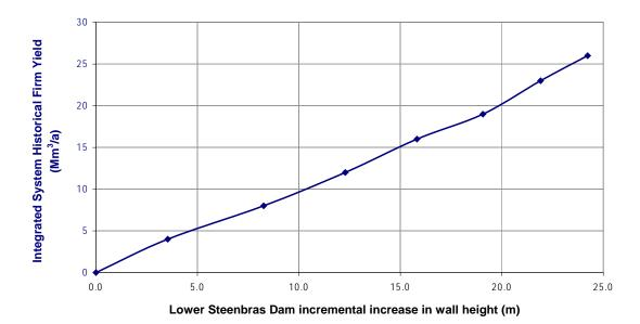
"i:lydro\400820\wrym\ib8\out\Steenbras Scenarios.xls" sheet "Plot wall heights Lower Integ" Figure 2: Increase in the historical firm yield of the integrated system from raising the Lower Steenbras Dam
